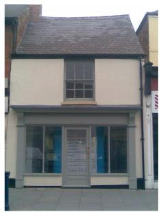
The former Arbon and Watts toy shop on Sherrard Street was re-roofed in natural slate and the upper floor aluminium double glazed window replaced by a traditional Georgian timber double hung box sash window. The aluminium shop front has also been replaced with a traditional timber frontage with central door. A traditional hand painted sign will complete the transformation once new tenants are found.
